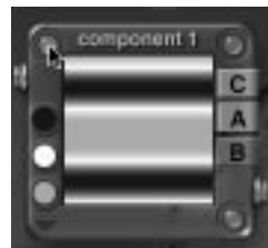
The three buttons along the outside of a component window let you display the Noise, Phase and Filter palettes.
