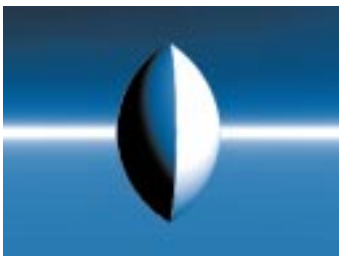
Boolean Intersection is performed by grouping a Positive object with an Intersecting object.
